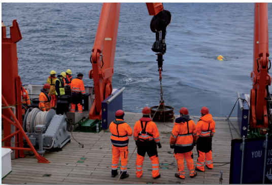
Deployment of an oceanographic mooring during the expedition MSM54 with RV MARIA S. MERIAN into the Labrador and Irminger Sea. These moorings are used for the long-term observation of ocean circulation. Photo credit: Arne Bendinger/ GEOMAR
