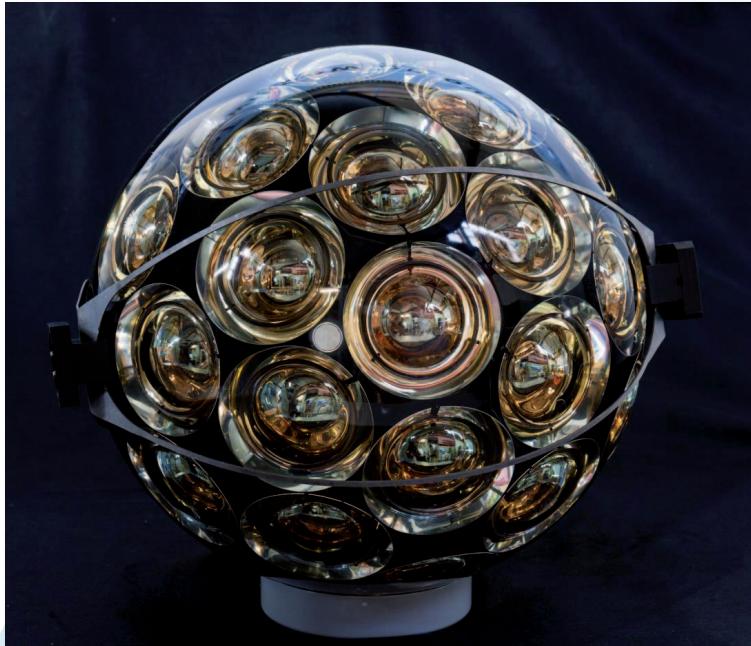
The KM3NeT optical module is a pressure resistant glass sphere housing 31 photosensors that will detect the faint flashes of light originating from interactions of neutrinos in the abyss of the Mediterranean. The full infrastructure will house about 6000 of these modules. The optical module is a Dutch design. Photo Credit: KM3NeT.
