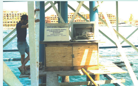
Mechanical tide gauge in operation at the southern end of the peninsula of Baja California, 1976. Photo credit: Modesto Ortiz-Figueroa, CICESE.
