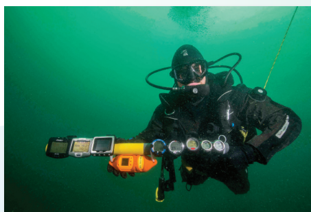
A scientific diver compares the performance of dive computers against that of a YSI portable CTD instrument. Photo credit: NFSD.
