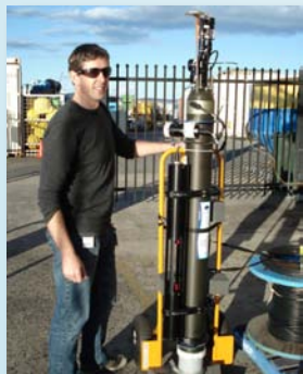
CSIRO Ocean and Atmosphere's Nick Hardman-Mountford testing one of the Bio Argo floats in Hobart. Photo credit: CSIRO
