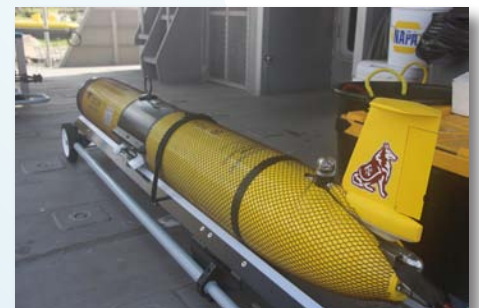
Several gliders and one autonomous surface vehicle will be deployed as part of the hypoxia monitoring experiment in summer 2014. Image credit: GERG, TAMU
