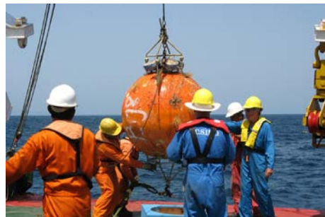
Deployment of Acoustic Doppler Current Profilers (ADCPs), instruments that measure the current speed and direction in the water column, in the Ombai Strait, 2006. Image credit: Scripps
