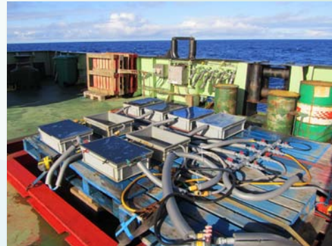
On-deck incubators for measuring primary production (G. Tilstone).
