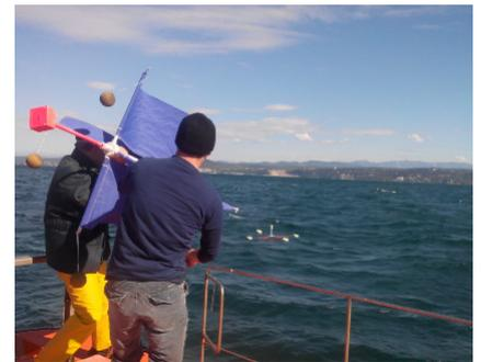
test deployment of one drifter at sea
